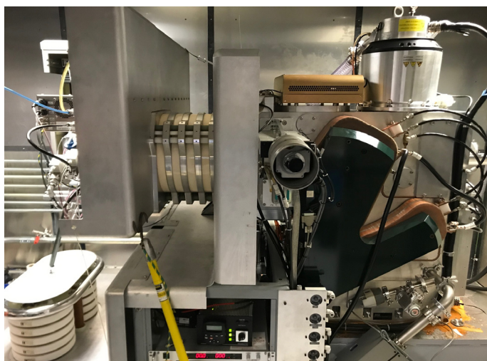
Ion Source Test Stand
